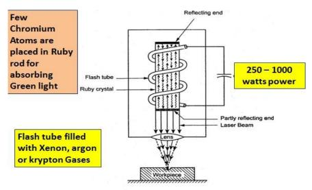
Schematic diagram of LBM
