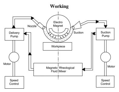
Fig. Magneto rheological fluid circulation system
