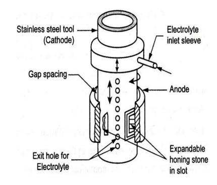
honing operations, except that they must resist the corrosiveness of the electrolyte. The honing stones are mounted on the tool body with a spring-loaded mechanism so that each of the stones exerts equal pressure against the workpiece.
