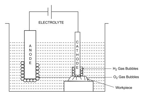
Fig. Electro chemical spark machining process
