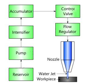
Reservoir: It is used for storing water that is to be used in the machining operation.
