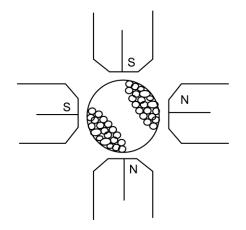
Fig. Magnetic abrasive finishing - internal surface
