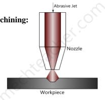
machining, metal removal rate increases with increase in velocity of abrasive particles.
