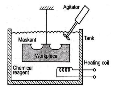
occurs in corrosion or as chemical dissolution of а metal. This controlled chemical dissolution will simultaneously etch all exposed surfaces even though the penetration rates of the material removal may be only 0.0025-0.1 mm/min.
