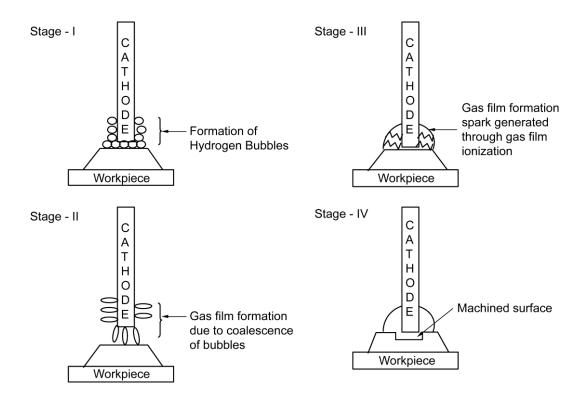
Fig. Stages in electro chemical spark machining
