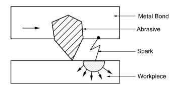
Fig. Formation of Spark in an Abrasive
