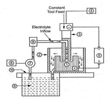
Workpiece, 2. Tank, 3. Tool (cathode), 4. Servomotor for controlled tool feed, 5. D.C. Power supply, 6. Electrolyte, 7. Pump, 8. Motor for pump, 9. Filter, 10. Reservoir difficult-to –machine materials. Difficult shapes can be made by this process on materials regardless of their hardness. A schematic representation of ECM process is shown in Figure. The ECM tool is positioned very close to the workpiece and a low voltage, high amperage DC current is passed between the workpiece and electrode.
