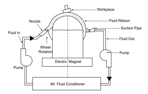
Fig. Magneto rheological finishing process
