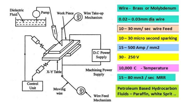
It also has work piece mounting table and a wire driver section. The wire driver section is use for moving the wire accurately at a constant tension. Another important part is the dielectric fluid (distilled water) supplier having constant specific resistance. Wire EDM has the following features -
