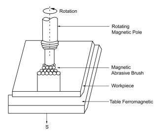
Fig. Magnetic abrasive finishing
