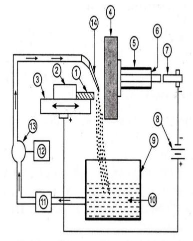
Workpiece, 2. Fixture, 3. Work table, 4. Grinding wheel,
