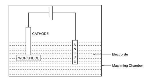
Fig. Principle of ECSM
