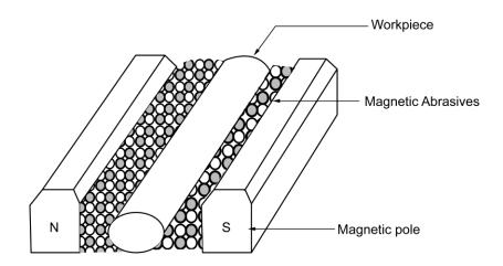
Fig. Magnetic abrasive finishing-cylindrical surface
