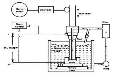
Schematic layout of EDM
